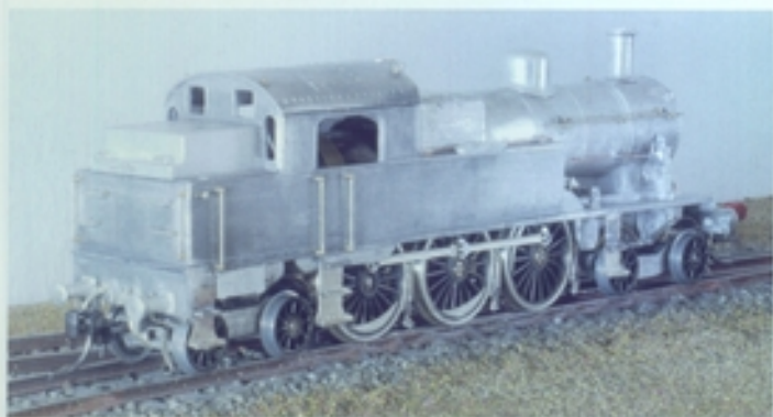
Above The bunker rear fits between the two main side tank and bunker sections, so the rivet line is unavoidably further in than it should be. Handrails and bunker steps are fixed with superglue; steps on the underside of the footplate are soldered.
