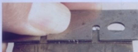
Left Making drop grab handles 2. The upright handle is then carefully bent flat, using a metal plate that is wide enough for leverage.
