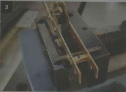
3 Levelling the frames in a machine vice with dummy axles. Once satisfactory, the threaded spacer screws are tightened and the chassis is soldered up permanently.
