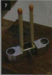
7 Preparing to low-melt solder the two separate cylinder castings onto a brass stretcher. Matchsticks allow the clamping force to be applied directly onto the cast-in frame mounting lugs to avoid any risk of misalignment during soldering.
