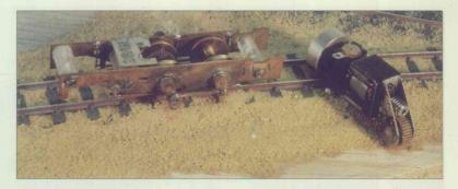
has its connecting rod pinned to the outside of the crosshead rather than the prototypically-correct inside position. It is also an idea to omit any retaining collar from the front crankpin for the same reason on a six-coupled loco, filing down the pin to the bare minimum to that capable of keeping the connecting rod in place.
