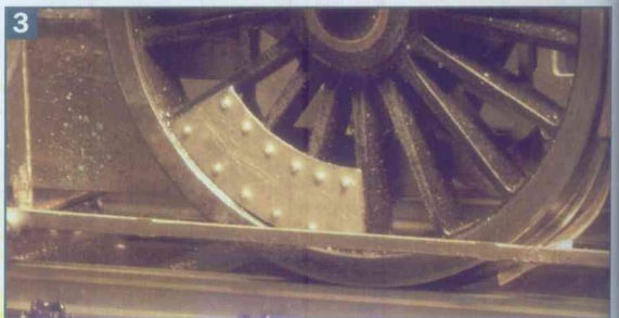
3 ▲ The coupled wheels' balance weights were fixed using superglue. Both wheel and etching were sanded to give the glue a key.
