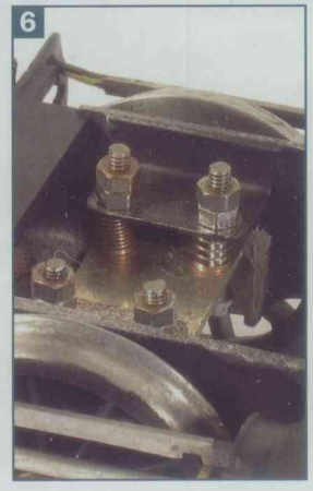
6 ▲ To ensure good adhesion, the leading axle is sprung using a quartet of Kadee coil springs. These push down upon a plate to which the axle is fixed, as seen in photograph 7.
